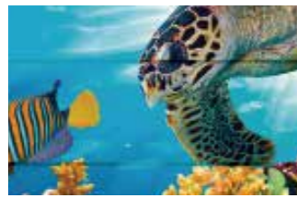
Overlap/Black streaks (Insufficient feeding amount)
