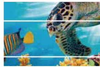
Gap/White streaks (Excessive feeding amount)
